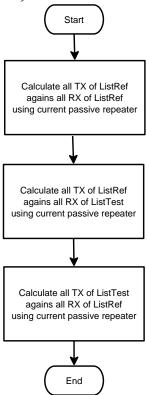
When PRX and PTX records are found the program starts calculations using passive repeater (function calcPTRCase). Flowchart of calcPTRCase (see diagram above) shows main three parts of calculations.
